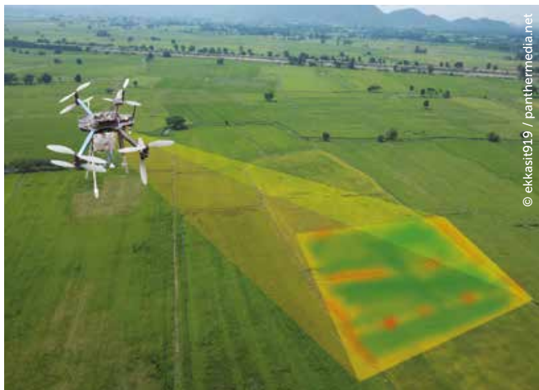
Left: Photonic sensors aboard automated drones are used for field and soil monitoring.
