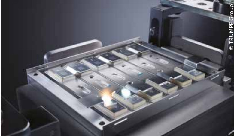
Left: Electrically high efficient and mechanically robust busbar connections with laser welding.
