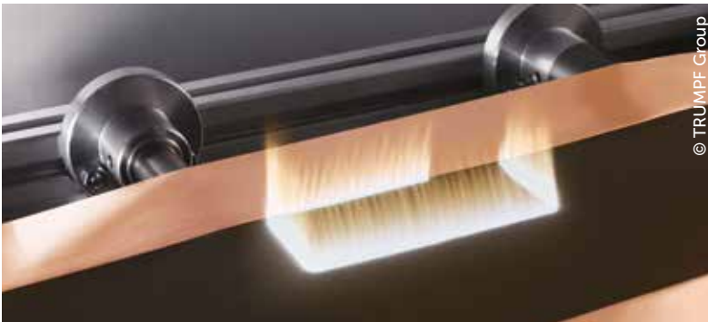
Left: Laser cutting of coated and uncoated electrode foil.
